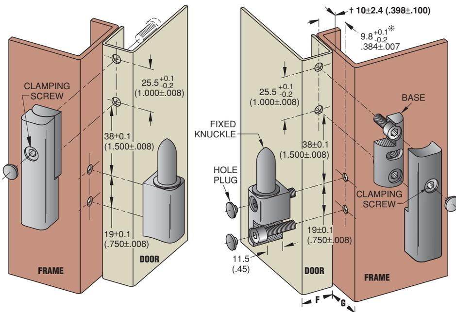
NOTES: Either **F** Dimension or **G** dimension must be less than 19.8 (.78) for the door to open a full 180°. \* Dimension will vary as † dimension is adjusted through its range. The door and frame design must allow for this variation.
