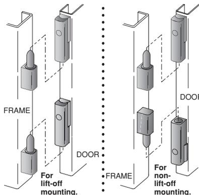
These hinges can be mounted on either side of door.
