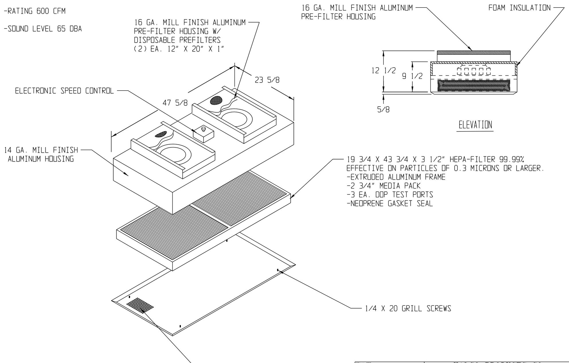
PERFORATED ANODIZED ALUMINUM PROTECTIVE GRILL WITH 1/8" DIA. HOLES ON 3/16" STAGGERED CENTERS ACCOUNTING FOR 40% OPEN AREA
