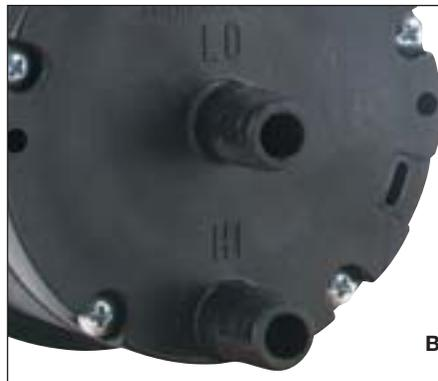
**A** The standard Minihelic® II gage is supplied with two barbed pressure taps molded into the rear housing of the gage. These connections allow easy, fast connection to the gage using  $\frac{3}{16}$ " I.D. rubber or plastic tubing.
