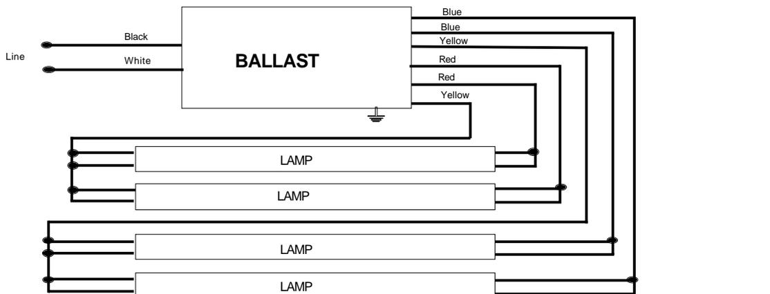
Note: For three lamp operation, cap any blue lead, insulate to 600 volts
