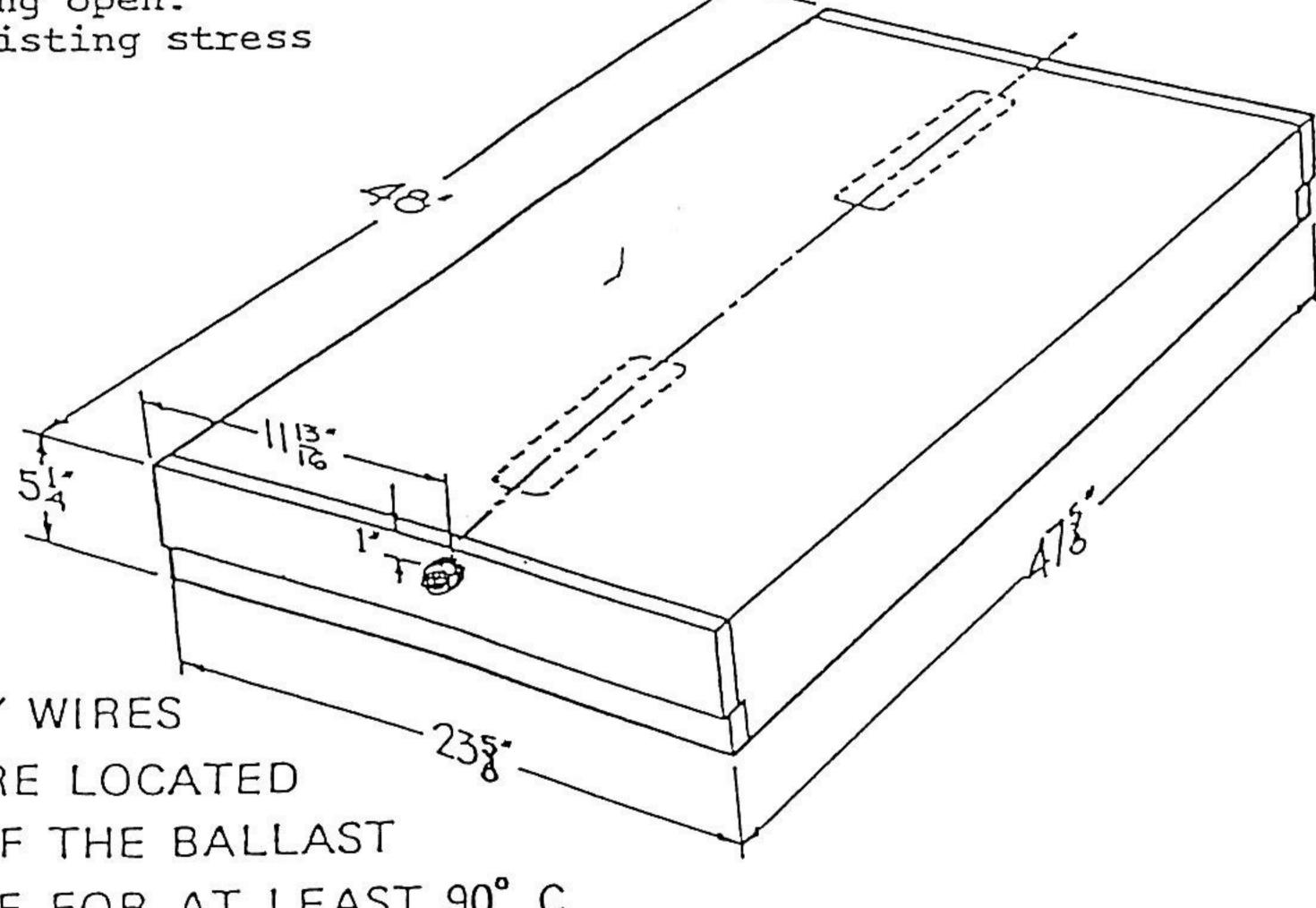
IF BUILDING SUPPLY WIRES OR POWER CORD ARE LOCATED WITHIN 3 INCHES OF THE BALLAST USE WIRES SUITABLE FOR AT LEAST 90° C.
