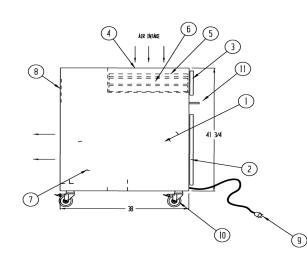
(1) I EA. IO-IDA DIRECT DRIVE BLOKER WITH 3/4 HP ECH NOTOR IIS YOLT, I PHASE 9.5 FLA CAPABLE OF 2000 CFM # 1.8" HC
