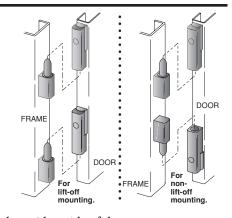
These hinges can be mounted on either side of door.
