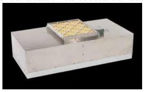
To keep this particulate matter from being recycled, both types of rooms use HEPA (high efficiency particulate air) filters. HEPA filters are manufactured from glass fiber, accordion-style pleated filters that can be up to 99.99% efficient in removing particles 0.3 microns and larger. For more stringent requirements, an ULPA (ultra low particulate air filter) filter may be used. An ULPA filter has the ability to remove a higher percentage of 0.3-micron particles than a HEPA filter.
